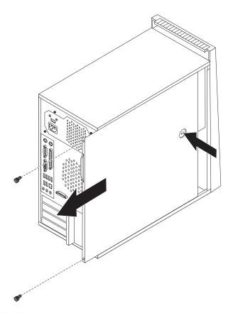
Figure 6. Removing the computer cover
